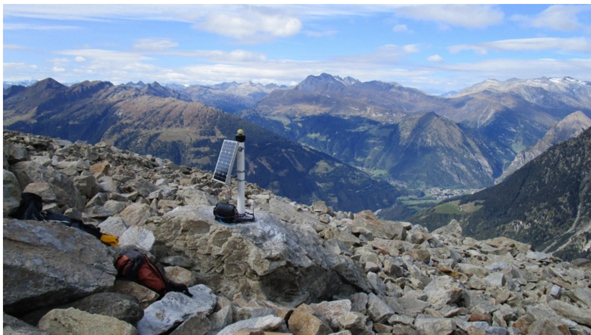
Figure 5.1. Permanent GNSS device on the Stabbio di Largario rock glacier (Ticino Alps). Photo: C. Scapozza.
