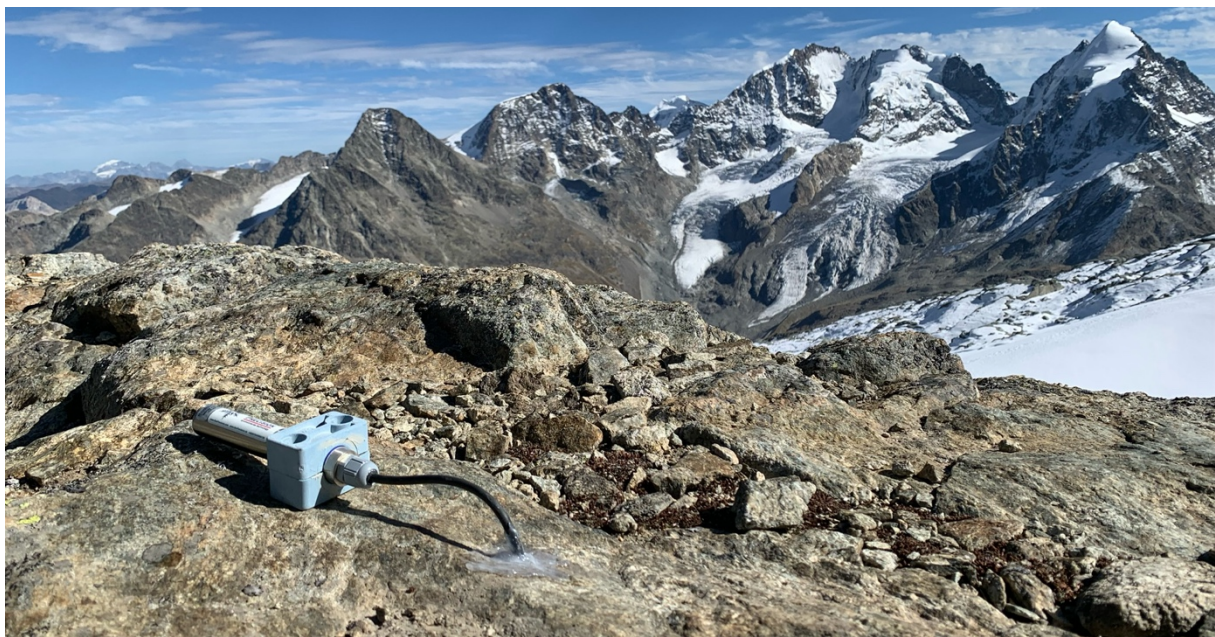
Figure 3.1. Miniature data logger recording ground surface temperatures in flat bedrock close to the Corvatsch summit station in the Upper Engadine at about 3300 m asl. Photo. M. Lichtenegger.
