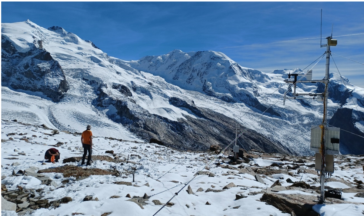
Figure 4.1. Electrical Resistivity Tomography (ERT) monitoring in September 2023 at Stockhorn. Photo: C. Hilbich.
