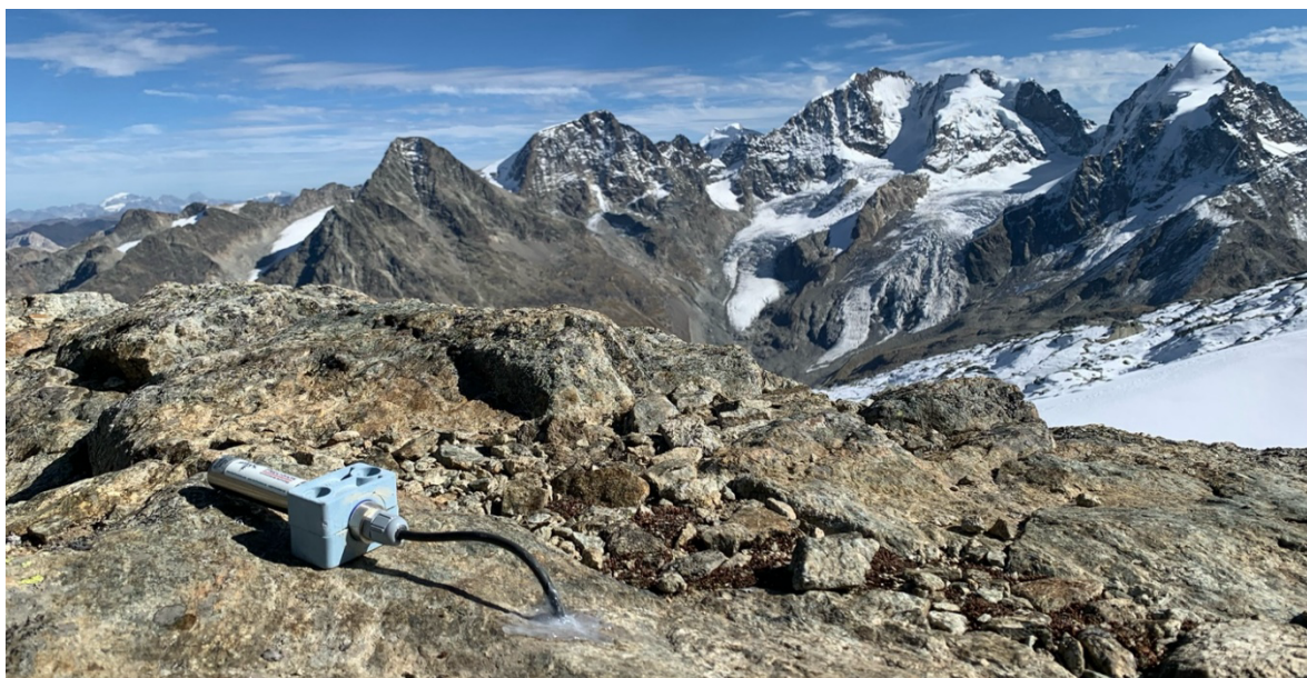
Rock surface temperature logger installed at the top of Piz Corvatsch in the Engadin at 3300 m asl. Elevation. Picture: Matthias Lichtenegger.
