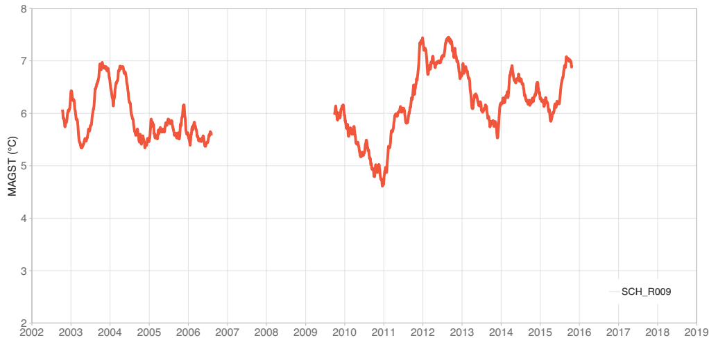
Figure A.20: Running annual mean of ground surface temperature time series measured at the site Schilthorn in near-vertical rock. Time series were gap-filled using the method by Staub et al. (2017) and only time series with at least 90% of data were selected. The thick red line is the mean of the individual loggers.
